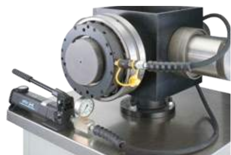
Mounting on adapter sleeve with a hydraulic nut
